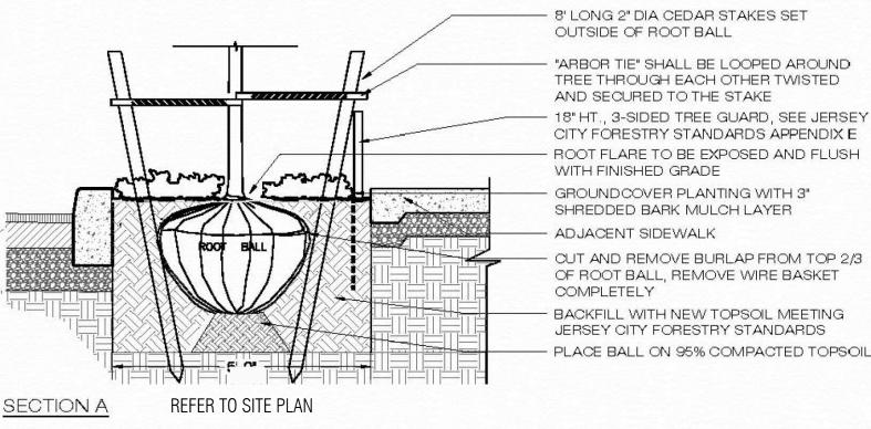
"ARBOR TIE" SHALL BE LOOPED AROUND TREE THROUGH EACH OTHER TWISTED AND SECURED TO THE STAKE 18" HT., 3-SIDED TREE GUARD, SEE JERSEY CITY FORESTRY STANDARDS APPENDIX E ROOT FLARE TO BE EXPOSED AND FLUSH
